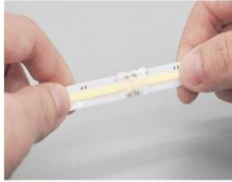
After complete the insert, also make sure both ends of led strip are tightly connected.
